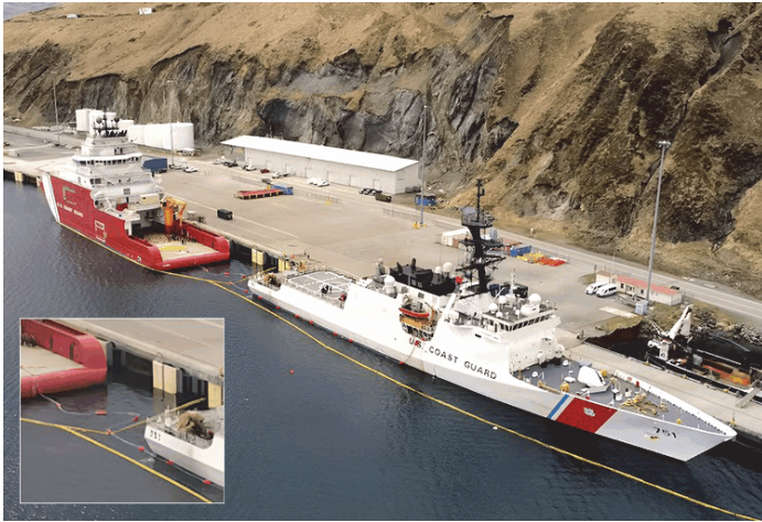
Figure 8. USCGC Storis (WAGB 21) left, and USCGC Waesche (WMSL 751) conducting a refueling exercise pier side at Dutch Harbor, Alaska, on 1 May 2026. Inset shows the small line (note red floats) passing fuel from Waesche to Storis.
