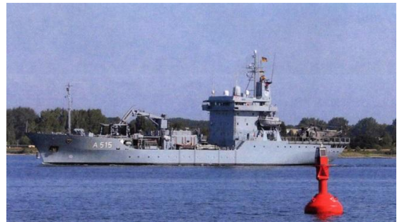
Figure 4: A515 MAIN, shown here entering Kiel harbor, is an ELBE-class tender modified to support the six Type 212A subs. Displacing 3,600 tons, it is the only tender of the German Navy dedicated to this task.
