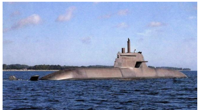
Figure 2: German Type 212A submarine U32 in Eckernförde Bay, unknown date. The smoothly faired transitions from the hull to the sail significantly improve the boat's stealth characteristics. The X-shaped rudders are just visible at the stern.
