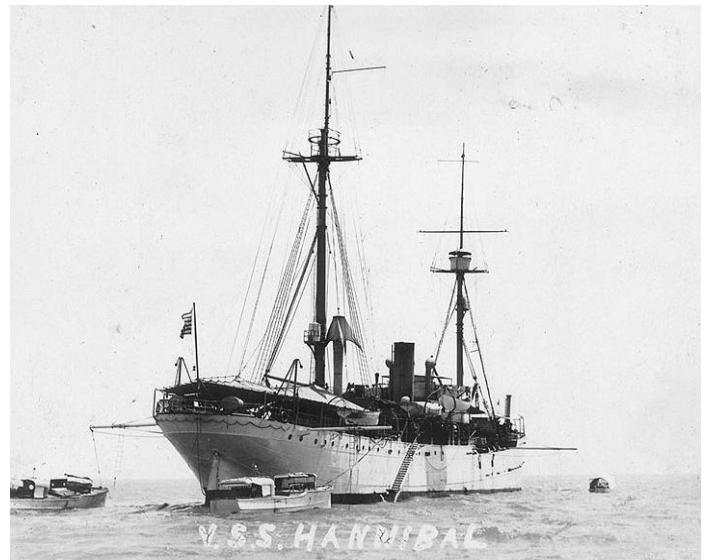
USS HANNIBAL (AG 1) at work off Cuba in the 1920s. HANNIBAL served much of her USN career as a hydrological survey ship. Her survey launches can be seen secured to boom forward; two more were secured at the stern. (photo US Navy)
